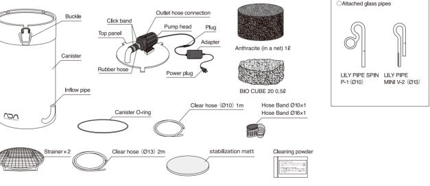
①Unlock the Buckle, open the Top panel, and take out the upper Strainer and Anthracite in a net from the Canister. ※Be careful not to hurt your nails when unlocking the Buckle. ②Take out the Anthracite from a plastic bag, keeping the Anthracite in the net, and wash it with water or warm water to take the fine powders away.
