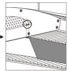
①Hold the shade with its coated surface outside and reflecting surface inside. Insert the mounting brackets into the gap between the outer plate of the Solar RGB main unit and the outermost radiation fin. ②Insert the mounting brackets securely until a click is heard and the claws fit into the hole on the outer plate of the Solar RGB main unit
