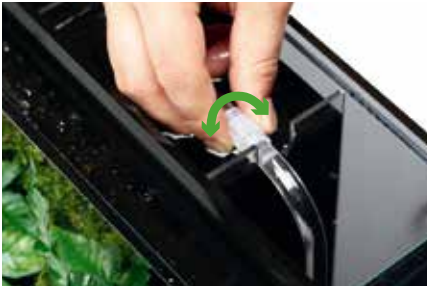
The flow rate controller maintains the optimum water surface level. The flow rate controller changes the flow rate of the water from the pump in the filter section and maintains the optimum water level in the cascade spillway.
